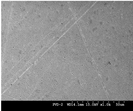
Figure 6. Surface of DLC films on head by RFMSD (1000 ×)
