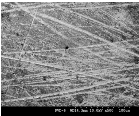
Figure 8. Worn surface of head by RFMSD (500 ×)
